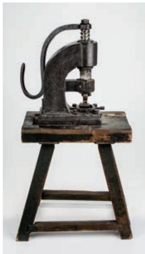
FIG. 3. The first type of special pressing instrument for metal jewelry. Manufactured by Kajetan Schier, Dalešice. 1840–1852. Pressing instrument: H. 46 cm, W. 30 cm. MSB Collection, N109. (Photo: Aleš Kosina)
