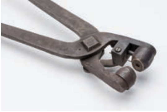
FIG. 2. Metal pressing pliers. Jablonec area (detail). After 1900. L. 43 cm. MSB Collection, N516. (Photo: Aleš Kosina)
